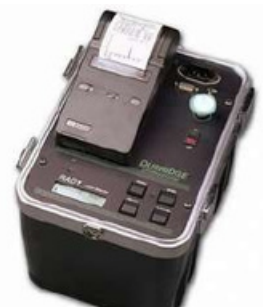
Radon Gas Monitor DurrIDGE RAD7
